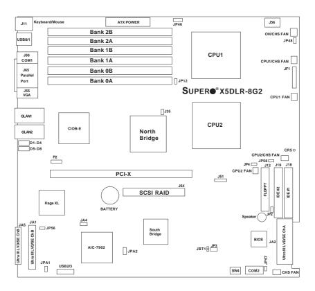
**Note:** the X5DLR-8G2+ has the same layout but has 1) no parallel (printer) port and 2) a standard PCI-X slot.
